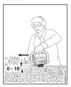
Hold the cutter bar at an angle of 0° to 10° as you swing the hedge trimmer horizontally.
