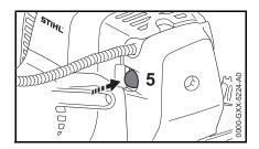
Press the manual fuel pump bulb (5) at least five times – even if the bulb is already filled with fuel.
