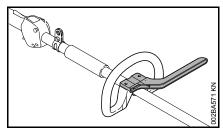
A barrier bar may have to be mounted to suit the tool you intend to use – see "Approved Combinations of Cutting Attachment, Deflector, Handle and Harness".
