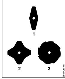
The cutting edges of the grass cutting blades (1) and (2) may point in either direction – these cutting attachments must be turned over regularly to reduce one-sided wear.
