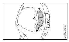
The throttle set wheel (4) enables the travel of the throttle trigger to be preset anywhere between idle and full throttle.
