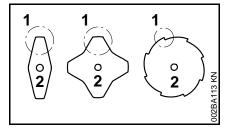
Resharpen the teeth (1) uniformly – do not alter the contour of the parent blade (2) in any way.
