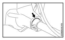
A vibration-absorbing rubber element is installed between the powerhead and the shaft. Have it checked in the event of noticeable wear or constantly increased vibration.
