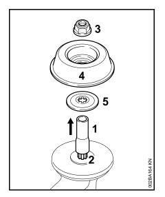
Depending on the cutting attachment, it may be necessary to use the nut (3), rider plate (4) and thrust washer (5).
