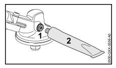
Check grease level after every 25 hours of operation and re-lubricate if necessary.
