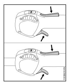
Depress throttle trigger lockout and pull the throttle trigger – the choke knob moves to the Run I position.
