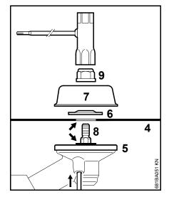
• Place the cutting attachment (4) on the thrust plate (5).
