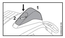
• Fit the cap (1), insert the screw (2) and tighten it down firmly.
