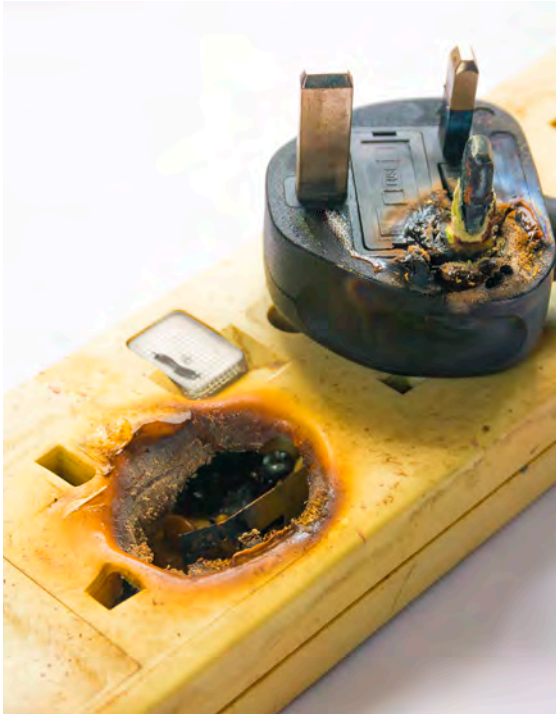
Figure 3: Damaged extension leads should be taken out of service immediately
