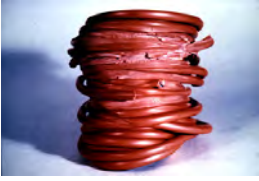
Figure 2: Wound extension cable showing overheating
