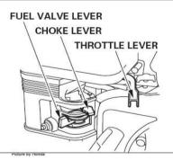
Pull the engine recoil handle slowly until it engages then pull hard and fast to start the engine.
