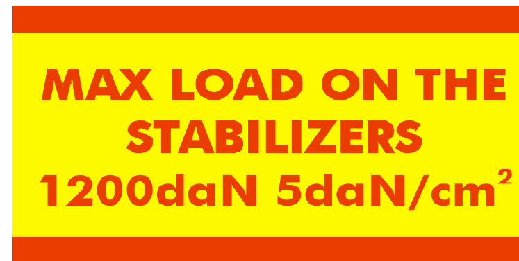
Picture 54: max load and specific pressure on the stabilizers
