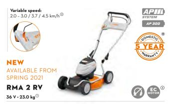
Lightweight and easy-to-manoeuvre mulch mower with a 46 cm/18" cutting width for medium-sized areas of lawn. Cut-height adjustment by axle, quick-fix quick-release tensioner and folding handlebar. Electric Vario wheel drive for comfortable work. The maximum working speed can be adjusted using a lever on the handlebar, with six levels available. For more information on features and technical details, see page 152. Working area covered with recommended AP 300 battery is 510 m<sup>2</sup>.
