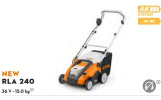
Compact cordless aerator for scarifying and combing smaller areas of lawn. Central adjustment of the working depth using a rotary switch on the housing, handlebar with 4-setting height adjustment, 34 cm working width, 16 blades. Includes scarifying blade, spring tine roller and 50-litre grass catcher box. For more information on features and technical details, see page 164. Working area covered with recommended AK 30 battery is 250 m<sup>2</sup>.
